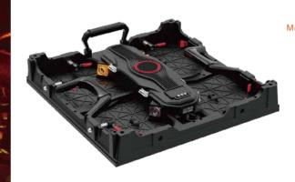
Uninterrupted Signal Transmission **Ensuring Consistent Performance** Dual Ethernet Port Backup Design, Providing Peace of Mind for Events
