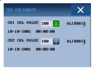
Figure 13-5 IBP Pressure Calibration Menu
