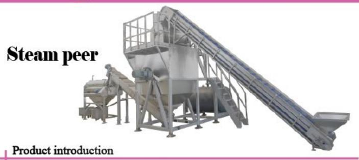
Steam peeling is the most efficient method of removing skin from fruit and vegetables. Lines processing between 1,000 kg/hr - 65,000 kg/hr can benefit from TINWING's steam peeling equipment, resulting in significant raw material and energy savings. TINWING offers a range of peeling solutions for French fries, and food processing lines for various root vegetables such as potatoes, carrots, sweet potatoes, red beets, celeriac, swedes, pumpkins, peppers, chillies, and many others.
