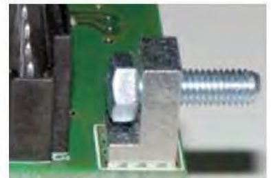
Angled power element for connecting the assembly with the housing
