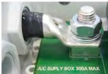
Press-Fit element for currents of up to 300 A
