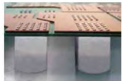
Press-fitting of power element: PCB with copper bar
