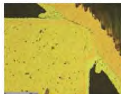
Continuous and extremely homogenous material transition between press pin and through-hole plating.
