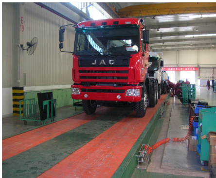
Truck Bottom drag chain assembly line and heavy truck front axle conveying system
