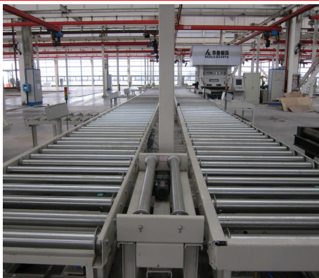
Ground material shuttle trolley transportation and brake hub air transportation system
