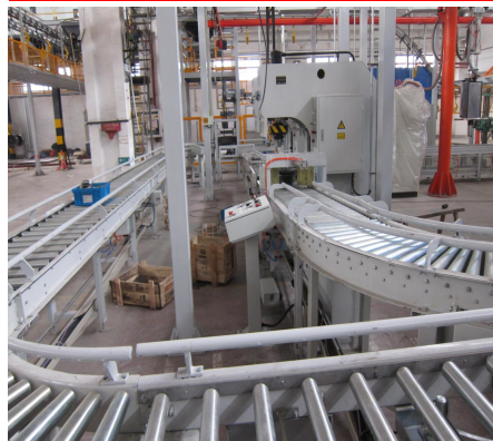
Ground material shuttle trolley transportation and brake hub air transportation system
