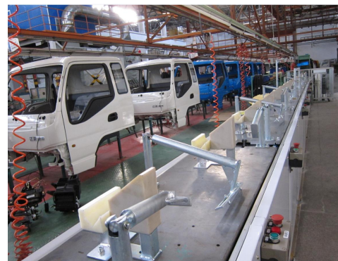
Truck hub turnover conveying system and truck instrument table conveying system
