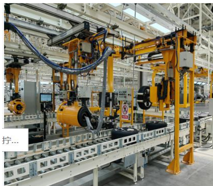
Line-side manipulator and custom high-position assembly line
