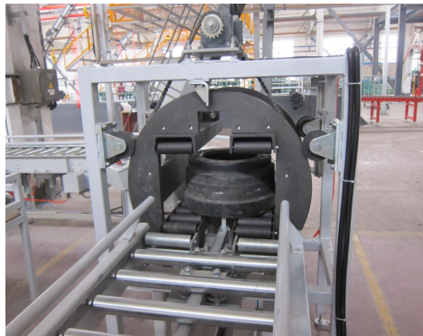
Truck hub turnover conveying system and truck instrument table conveying system
