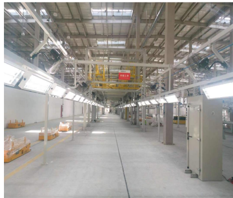
Line-side manipulator and custom high-position assembly line
