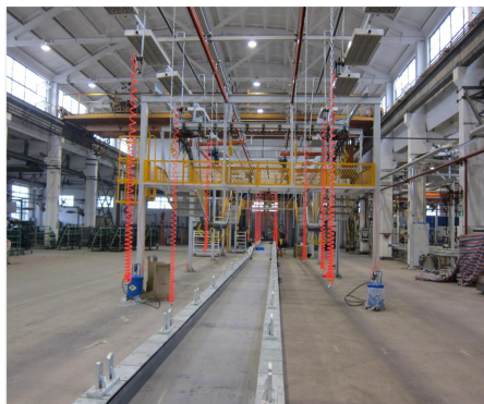
Truck Bottom drag chain assembly line and heavy truck front axle conveying system
