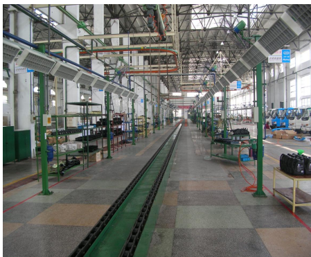
Truck Bottom drag chain assembly line and heavy truck front axle conveying system
