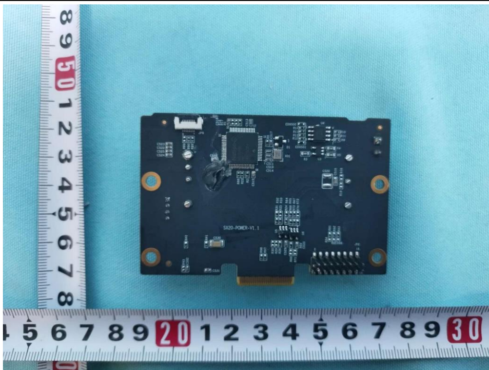
Solder side of Main board-2
