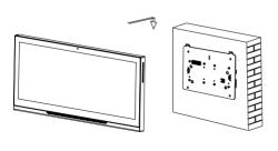
Align the holes on the back of the device with the hooks of the mounting box and clip in.
