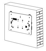
Pre-install 2x86 boxes in the wall, connect cables to the corresponding ports on the mounting box(please refer to the device wiring section). Fasten the mounting bracket to box by using screws.
