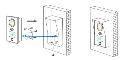
Use screws to fix the rain cover on the wall. Connect cables to the doorbell, fix the cover pad by screws. Mount the doorbell to the rain cover, use screw to fix it at the bottom side.
