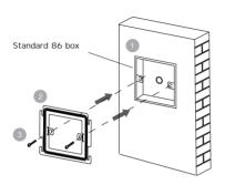
Pre-install standard 86 box in the wall, fasten the bracket to the box using screws.
