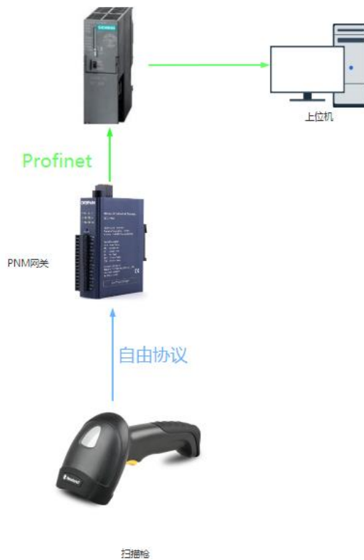
Topology of free port transparent mode
