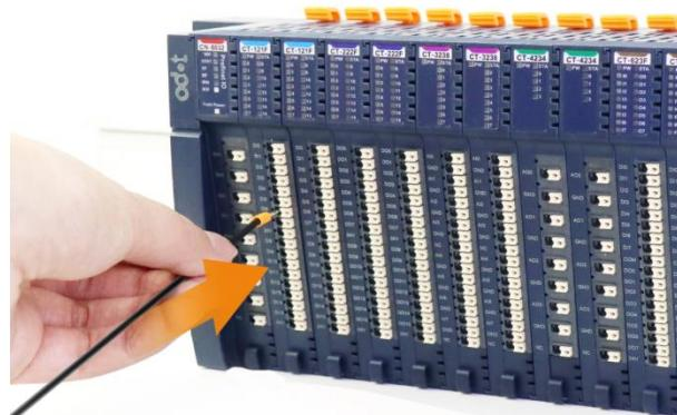
The module equips with a wiring fixed end for cable harness, which is used to fix the cable when the IO module is wired with multiple cables.
