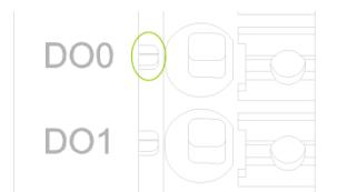
When the output signal of the output channel is valid, the corresponding channel indicator is on.
