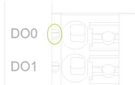
When output signal of output channel is valid, the corresponding field channel LED indicator is on.
