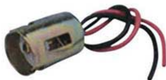
For GM signal/park/stop & tail flush-mounting snap-in double contact GM 5947900 lamp nos: 198.1016 1034.1154.1157. Fits 1-1/8" hole
