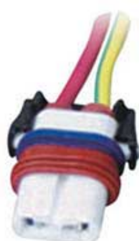
9006 Bulb Socket, ceramic
