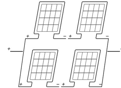
Tips: When it's series connection, the voltage is added, but the current is not changed; When it's parallel connection, the voltage is unchanged, but the current is added.
