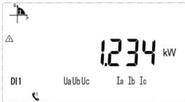
Current total power is 1.234kW
