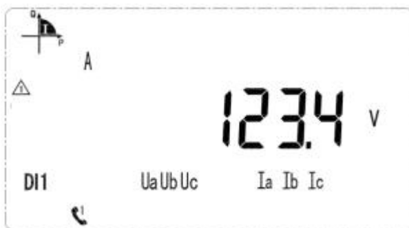
Voltage on A phase is 123.4V
