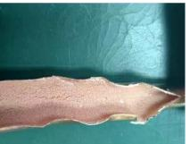
The internal sintering incorporates micro-nano thermal conductive materials, achieving a thermal conductivity 2 to 2.5 times that of copper powder and increasing capillary force by more than three times.
