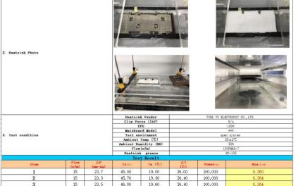
Actual test results: 100W: ambient temperature of 26 °C, thermal resistance of 0.264 °C/W, temperature rise of 26.4 °C Technology Study / Product case Liquid-Cooled
