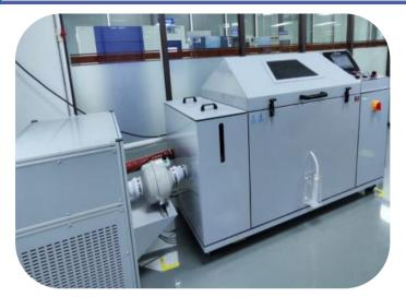
**Instrument Name**: Composite Salt Spray Test Chamber Parameter:
