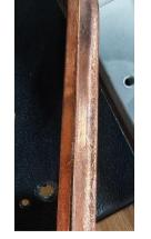
Standard flattened pipe: Side indentation s after roll-pressing
