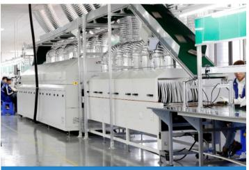
High-precision reflow soldering production line
