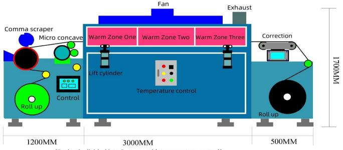
(Drying is divided into 3 stages with temperature control)
