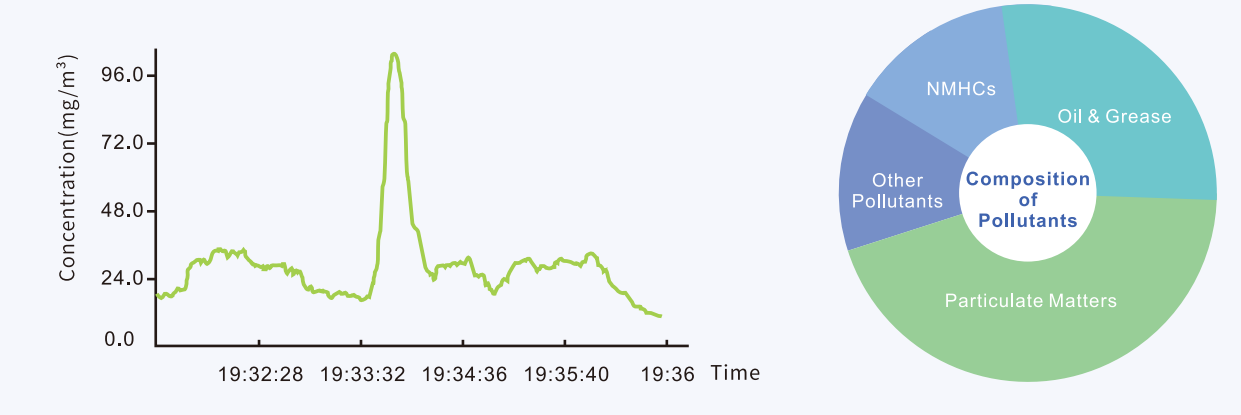
Concentration Curve of Smoke Particles Measured at a Barbecue Restaurant Reports show an Avg. 37mg/m³ & Max. 100mg/m³ concentration in such establishments
