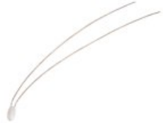
2.252K reusable temperature resistor
