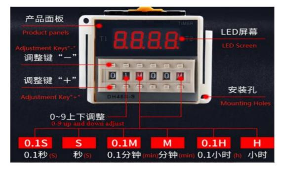
The opening and closing times of the electric valve can be adjusted as required, with the stopping time set in the right area and the working time set in the left area. General setting: stop time (closed) 10 minutes, working time (open) 6 seconds. The working time and working condition can be adjusted, e.g. 10 minutes closed, 10 seconds open.
