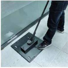
When activating the Shutter Magnet switch, do not use a metal hammer to strike it directly. Instead, it is advisable to press it down with the sole of your foot, applying your body weight. However, avoid lifting your foot and stomping down forcefully to prevent slipping and potential injury while stepping on it.
