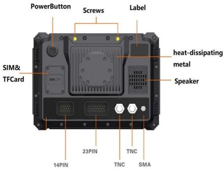
\*The default connector on the back is 14PIN+23PIN+2\*TNC+1\*SMA, it can be customized
