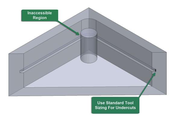
Undercuts should be carefully evaluated during the design phase to avoid unnecessary complexity and cost. Non-standard feature sizes may require expensive custom tooling, significantly increasing production time and expense—especially for low-volume manufacturing. Additionally, limitations in tool geometry restrict the achievable depth and location of undercuts, making shallow and easily accessible designs more practical.
