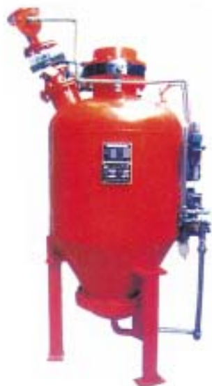
上引式仓泵 Ascending suction transport
