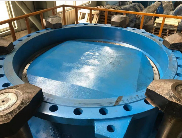
◆ Sealing test for forward and reverse direction
