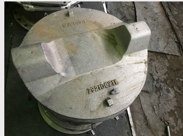
◆ Valve body and disc test specimen
