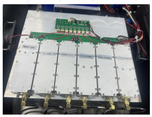
7. High temperature resistant, 50ohm semi-flexible cables, low loss, low insertion loss, connectors can be up to 6G.
