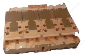
Gan power tube internal matching amplifier Rectangular waveguide power synthesis High-speed pulse power supply drain modulation Power-on/power-off timing protection function
