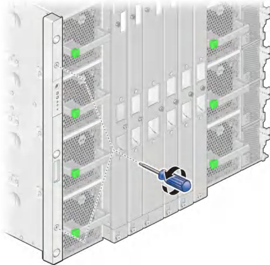
6. With the faceplate removed, remove the No. 1 Phillips screws to free the indicator panel from the chassis.
