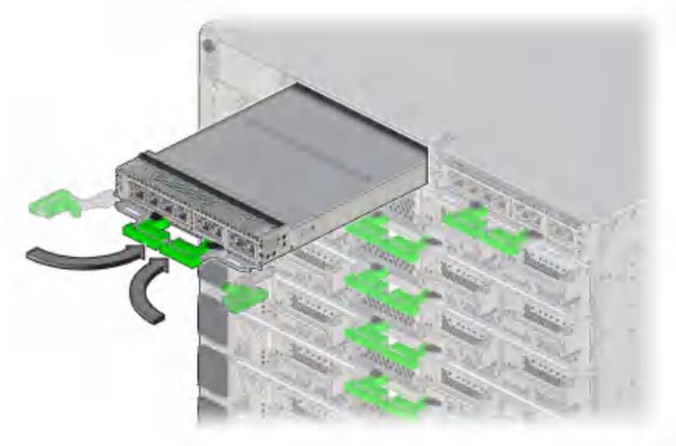
9. Carefully remove the component from the SP tray, using two hands, and avoid bumping the rear connectors.
