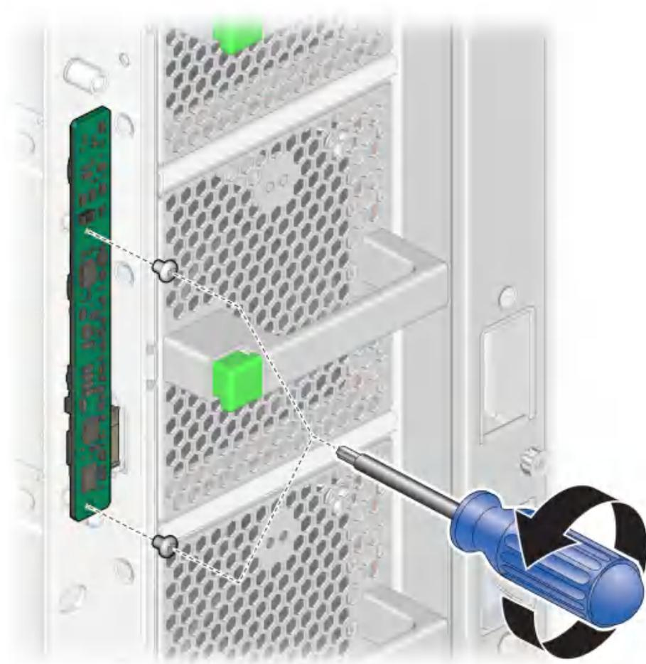
7. **Disconnect the small cable from the panel and remove the panel completely from the server.**
