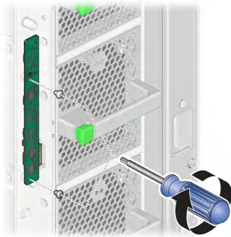
3. **Position the faceplate over the panel, install the Torx screws, and tighten the captive screws to secure the faceplate to the panel.**
