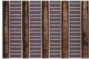
TS :260°C lead free reflow: 5X-0.8P
