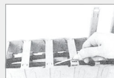
用螺丝刀作为杠杆把链盖封闭 Tighten the chain' cover by using screwdriver
