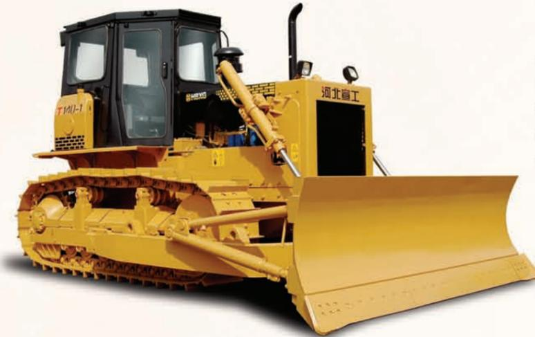
T140-1 Bulldozer is track-type model which utilizes semi-rigid suspension, mechanical drive and hydraulic control. It can be used in road building, hydro-electric construction, field modification, ports and mines development and other construction projects.
