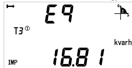
Current forward reactive total energy
