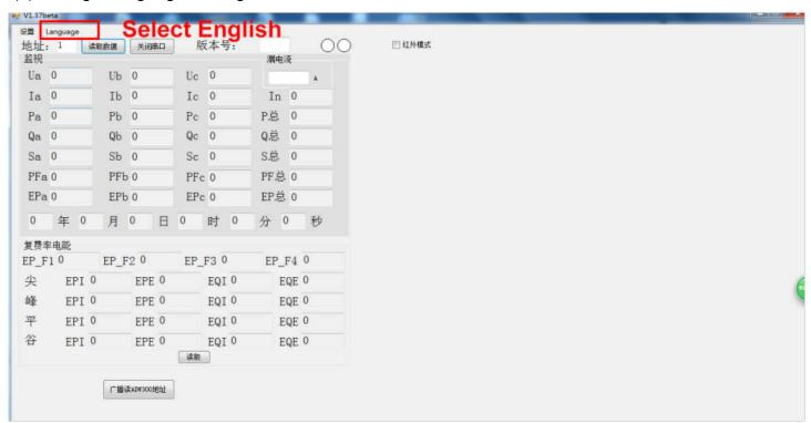
(6) Press "SET" and press" Serial Set" button and set the parameter as below (Note: COM No. should be as same as what we checked in the computer manager before)
