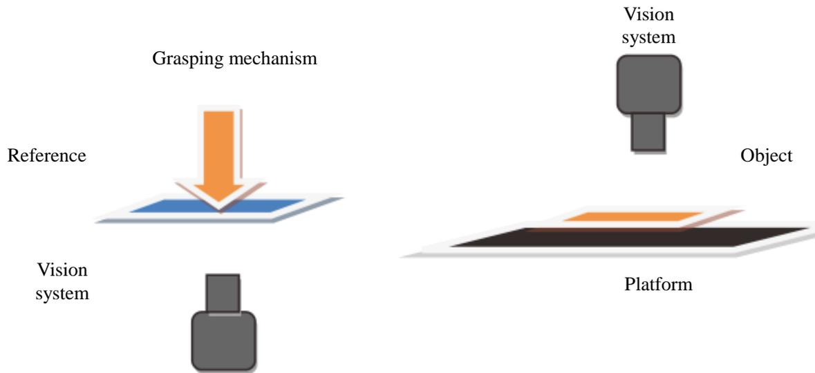
The vision system can use the template matching algorithms to calculate the coordinates  $(X, Y, \theta)$  of the reference. Similarly, it can also calculate the coordinates of the object.
