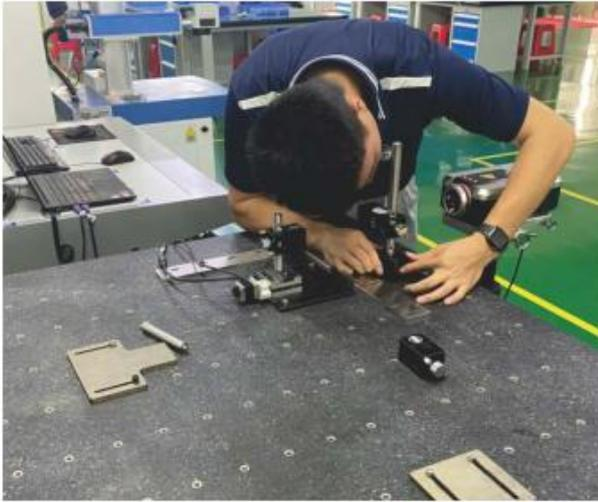
The laser interferometer can be used in combination with various refractors, reflectors, etc. to measure the linear position, velocity, angle, flatness, straightness, parallelism, and perpendicularity, and can also be used in calibration of precision machine tools or measuring instruments.
