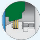
2. Eccentric three-layer composite metal sealing
