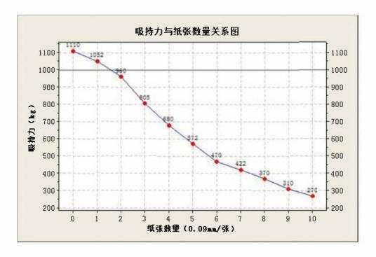
As illustrated in the figure above, the gap between the bottom of the Magnet block and the platform significantly influences the pull force of the shuttering magnet. Therefore, we recommend that customers conduct daily maintenance on the shuttering magnet.
