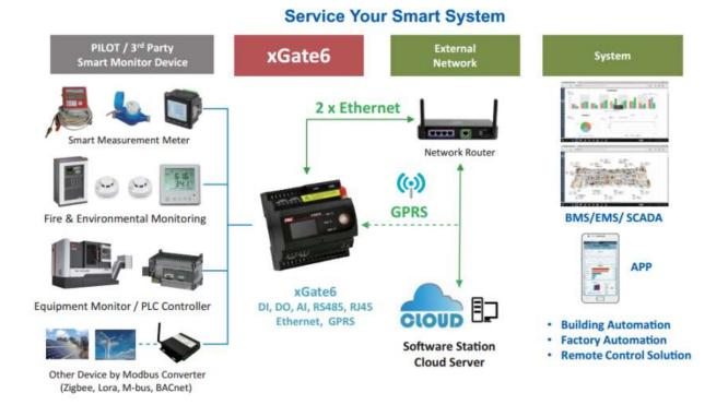
XGate6 intelligent gateway monitoring platform consist of 4 parts, they are Gateway module, Smart Device (intelligent power meter, smart power supply, etc),
